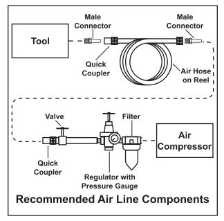
Attach an air hose to the compressor's air outlet. Connect the air hose to the air inlet of the tool. Other components, such as a connector and quick coupler, will make operation more efficient, but are not required.
